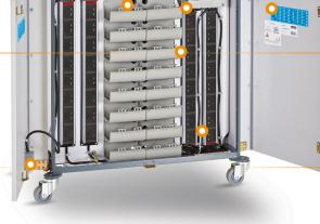
Device adaptors plug into 2x10-way power strips.
